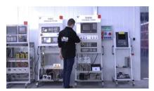
We have test stands developed by us, thanks to which we check whether the device is operational. They make sure that SIEMENS 6ES5374-1FH21 is repaired.
