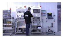
We have test stands developed by us, thanks to which we check whether the device is operational. They make sure that SIEMENS 1FT6062-6AF71-3EA2 is repaired.
