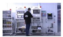
We have test stands developed by us, thanks to which we check whether the device is operational. They make sure that HEIDENHAIN ROD320.005-2500 is repaired.
