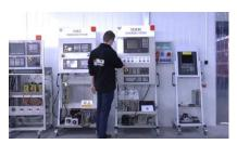
We have test stands developed by us, thanks to which we check whether the device is operational. They make sure that SIEMENS 6SL3224-0BE13-7UA0 is repaired.
