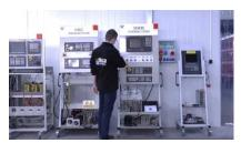
We have test stands developed by us, thanks to which we check whether the device is operational. They make sure that SIEMENS 6SL3211-0AB11-2BA1 is repaired.
