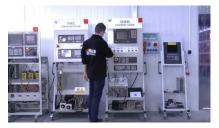
We have test stands developed by us, thanks to which we check whether the device is operational. They make sure that FANUC A06B-2212-B402#0100 is repaired.
