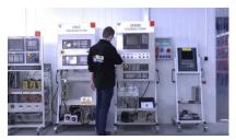
We have test stands developed by us, thanks to which we check whether the device is operational. They make sure that PERSKE FRLCS71.12/2 is repaired.
