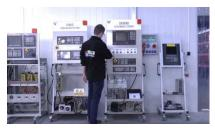
We have test stands developed by us, thanks to which we check whether the device is operational. They make sure that HIRATA HNC-D580-6 is repaired.
