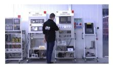
We have test stands developed by us, thanks to which we check whether the device is operational. They make sure that INDRAMAT DAA01.1 is repaired.
