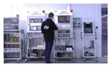
We have test stands developed by us, thanks to which we check whether the device is operational. They make sure that SIEMENS 6ES5095-8MA01 is repaired.
