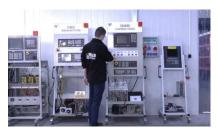
We have test stands developed by us, thanks to which we check whether the device is operational. They make sure that SIEMENS 6ES5453-4UA12 is repaired.
