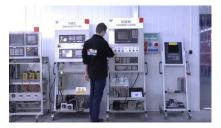
We have test stands developed by us, thanks to which we check whether the device is operational. They make sure that FANUC A06B-1431-B123#0121 is repaired.
