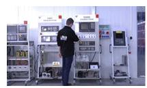
We have test stands developed by us, thanks to which we check whether the device is operational. They make sure that KONTRON CP306-V is repaired.
