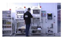
We have test stands developed by us, thanks to which we check whether the device is operational. They make sure that LENZE SD250 is repaired.
